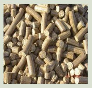
proper shaped briquette. The process consists of crushing, compressing and drying the final end product to increase their life span and efficiency.
